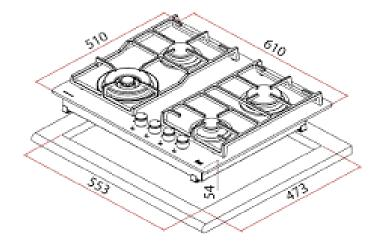
ATTENTION: Cut hole must be with round corners in order to avoid cracking on the counter-top.
